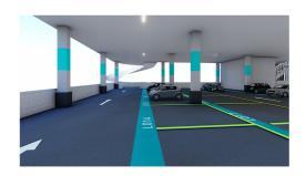
POLYDEC®CP system consists of multi-layered coats designed to provide total protection to the sub-floor. The system is solvent-free, low VOC and results in a water-tight, tough, anti-skid surface topped with a solvent-free UV stable PU coat to provide excellent film strength and scratch resistance.
